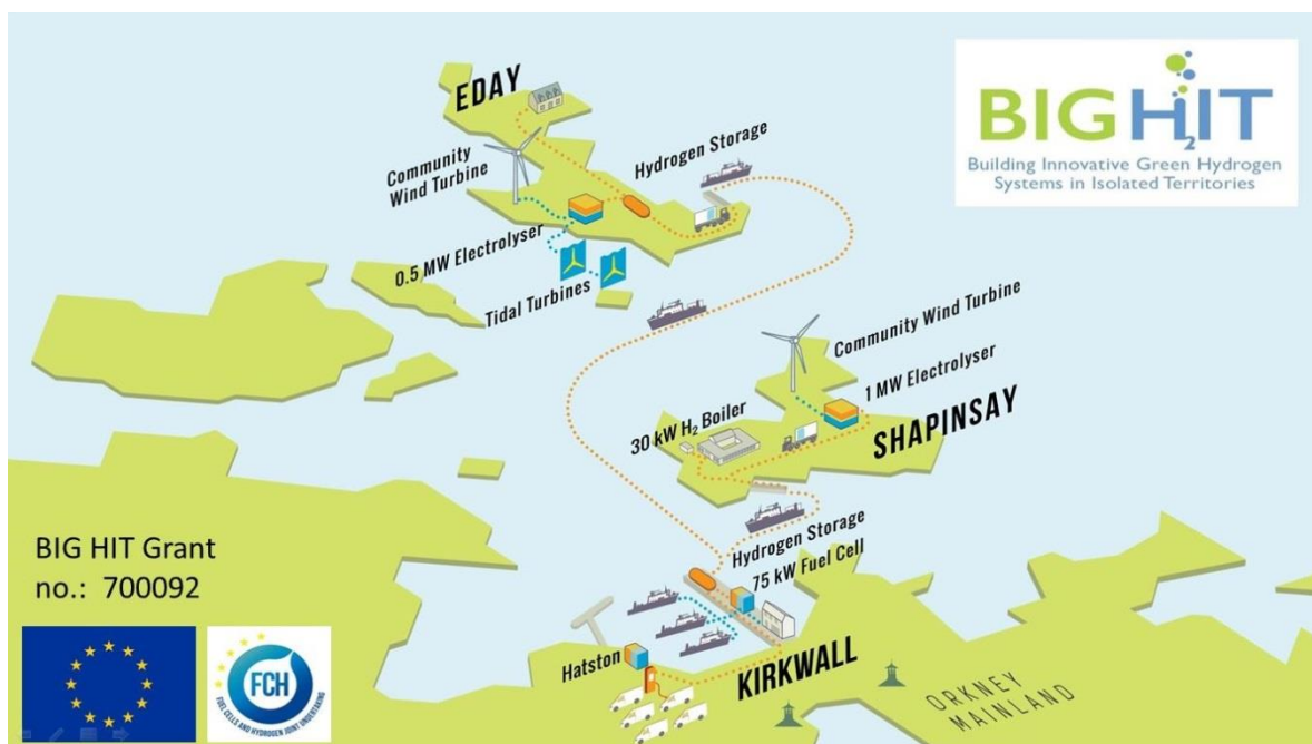
Figure 39: Overview of the BIG HIT project on the Orkney Islands
