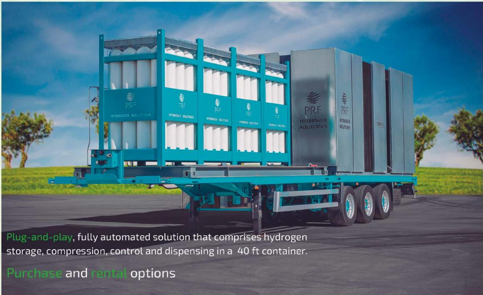
Plug-and-play, fully automated solution that comprises hydrogen storage, compression, control and dispensing in a 40 ft container.
